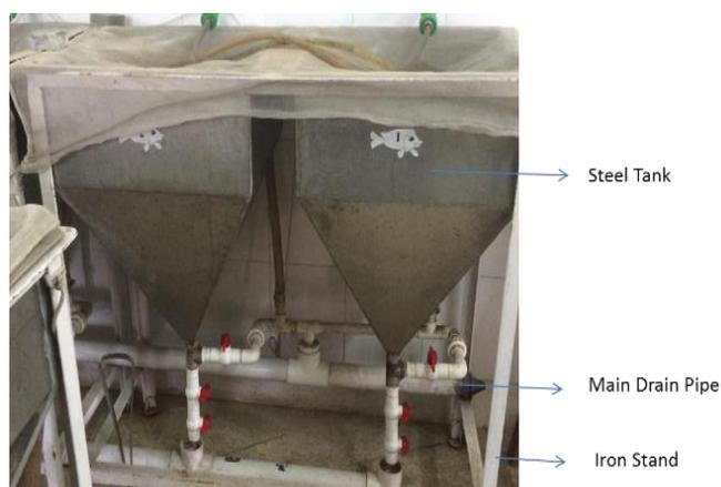
Figure 1: Modified UA system showing the steel tank and main pipe
