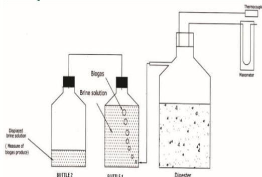
Figure 3: Schematic Diagram of the Water-Displacement-Method
