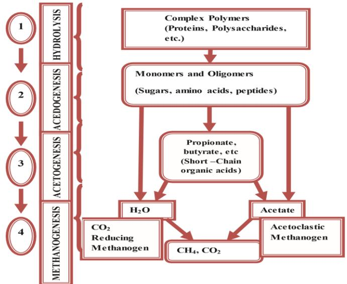
Figure 2: Four basic steps involved in biogas production
