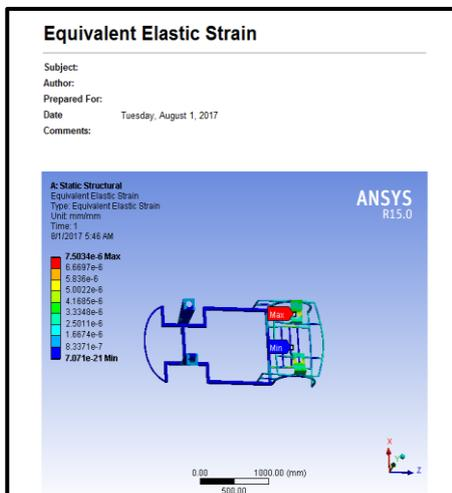
Figure 11: Equivalent Strain of chasis on ANSYS
