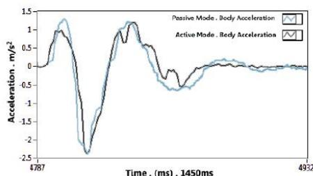
Figure 15: Experimental results for body acceleration in active and passive modes during 1450 ms test.
