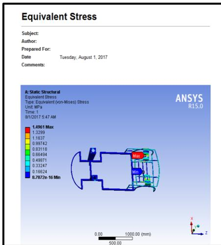
Figure 10: Equivalent Stress of chasis on ANSYS
