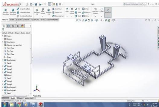
Figure 2: Design of chassis frame on SolidWorks
