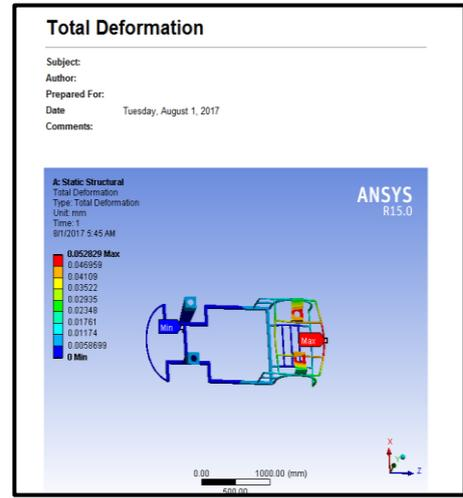
Figure 12: Total Deformation of chasis on ANSYS
