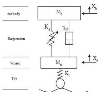
Figure 3: Free Body Diagram of Active Air Suspension
