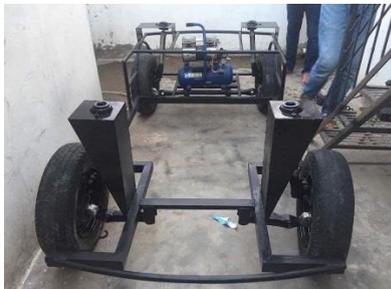
Figure 1: Active Air Suspension Unit
