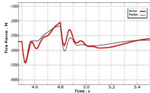
Figure 16: Diagram of tire forces in passive and active simulation test
