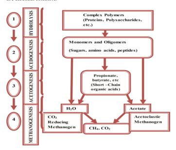
Figure 2: Four basic steps involved in biogas production
