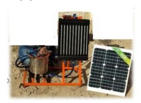
Figure 1: Showing portable biogas reactor
