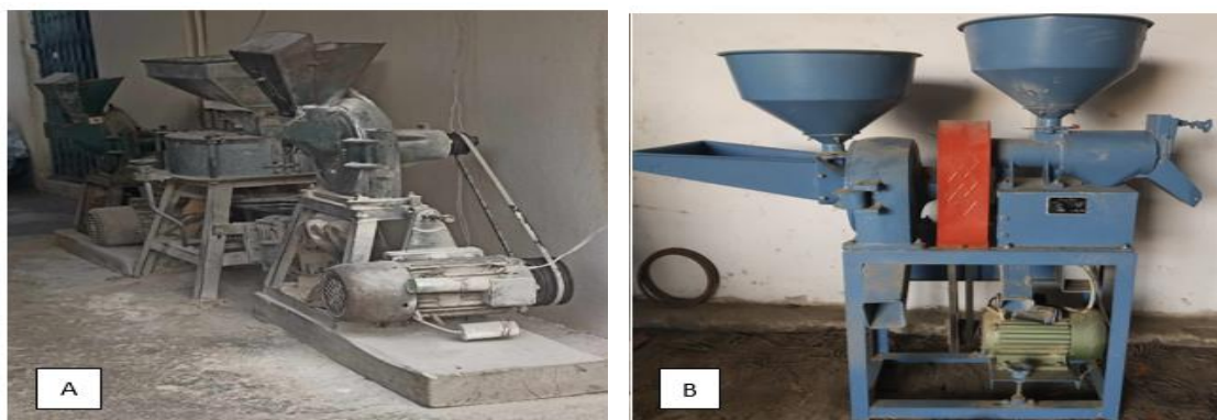
Figure 8: Small scale grain processing center in rural area (A) and Combine mill (B)
