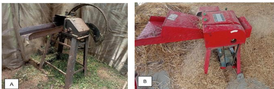
Figure 6: Chaff Cutter (A-fly wheel type and B-drum type)
